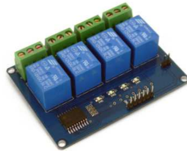
Figure.4 Four Channel 12v Relays
