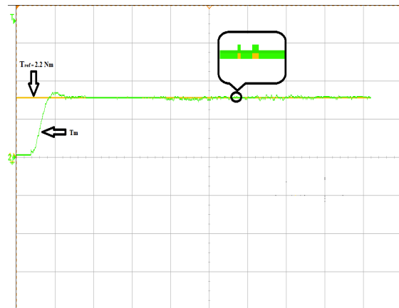
Figure 13 Torque Waveform For 100% Loading(X-Axis: Time In S, 1 Div= 10s, Y-Axis: Torque In Nm, 1 Div= 1.46 Nm)
