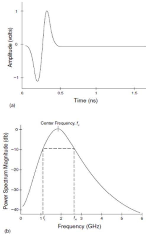
Figure 4: A 500 Picoseconds Gaussian Monocycle In (A) The Time Domain And (B) The Frequency Domain
