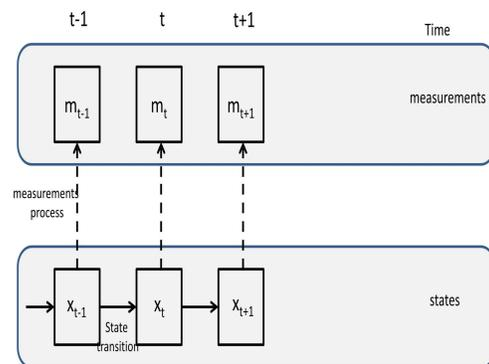
Figure 5: State Transition And Measurement Process In Particle Filter
