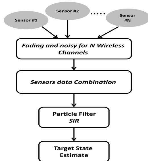
Figure 7: Structural Framework Of The Proposed Indoor-Outdoor Positioning System
