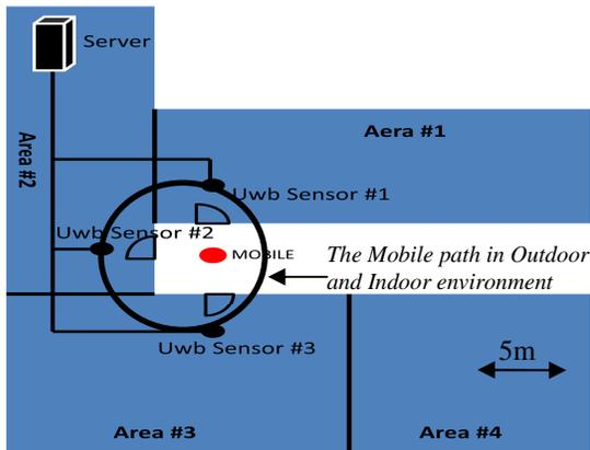
Figure 8: Plan Of The Laboratory, Including The Location Of The UWB Sensors
