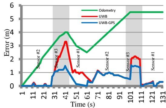
Figure 9: Localization Error For The Three Situations Along Two Loops
