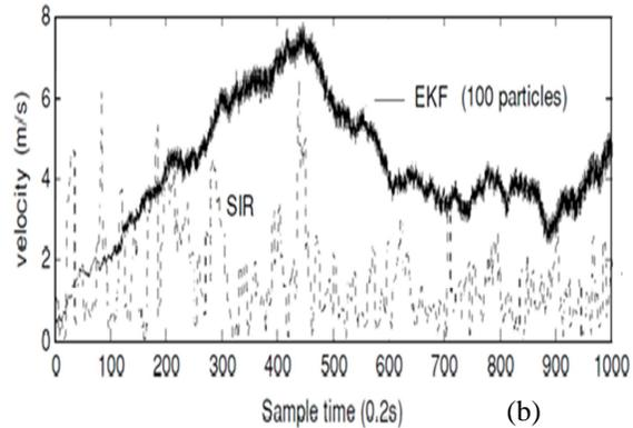
Figure 6: Comparison Between The SIR And The Extended Kalman Filter Concerning The Position (A) And Velocity Errors (B).
