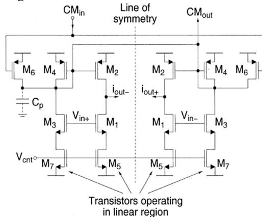
Figure 9. Schematic of the proposed differential transconductance [34].
