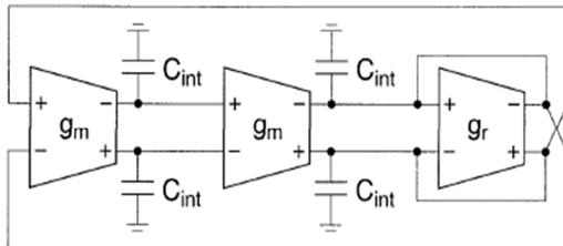
Figure 7. Fully differential two integrator loop Gm-C filter [34].
