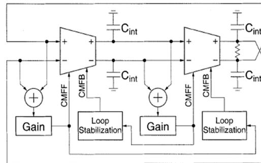
Figure 8. Two integrator loop transconductance with both CMFF and CMFB [34].
