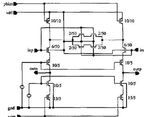
Figure 13. Unit transconductor element.
