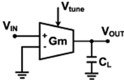
Figure 2. Typical Gm-C configuration [26]
