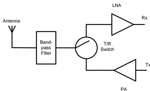
Figure 1. Bandpass filter at the transceiver front end
