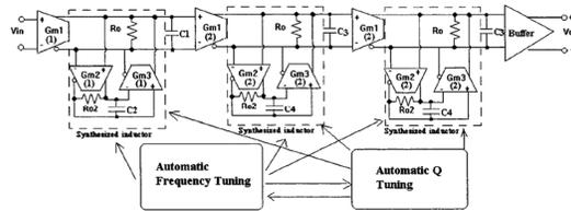
Figure 4. Three bi-quad stages of band pass filter [32]
