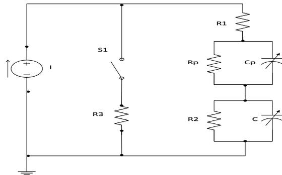
Figure 2: The Basic Circuit Model Of The Super Capacitor (EPOCS)
