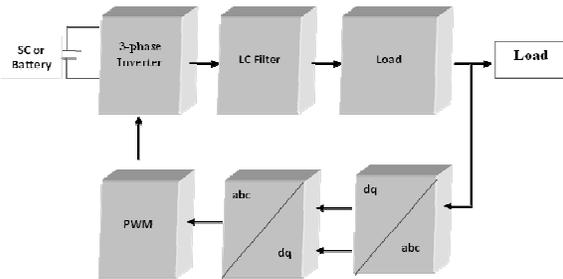
Figure 1: Model Layout Of Whole Proposed System
