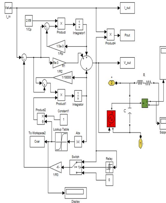
Figure 3: Simulink Model Of SC
