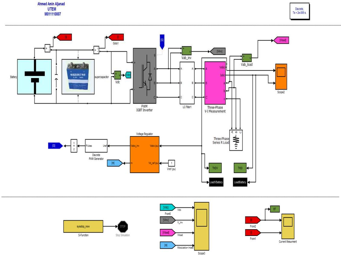
Figure 10: The Schematic Diagram Of The Whole System
