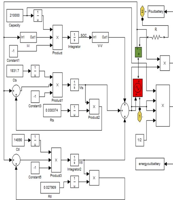
Figure 5: Simulink Model Of Battery
