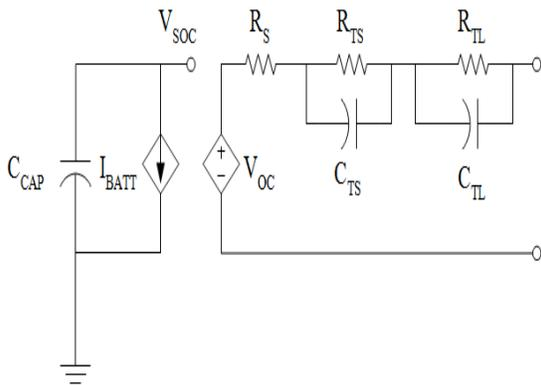
Figure 4: Circuit Model Of Battery
