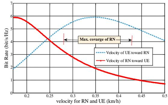
Figure 11 Bit rate change with the change in movement for both the UE and RN
