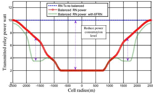
Figure 13. Saving transmitted power of MRN over cell radius
