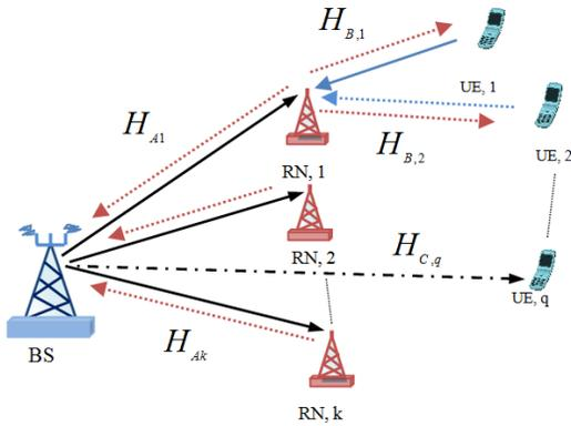
Figure 3 Half-duplex Relay scheme
