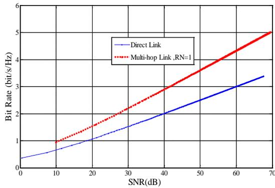
Figure 8. Bit rate and SNR enhancements between the direct and relay links
