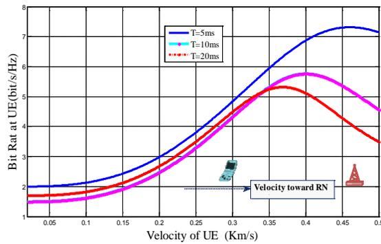
Figure 9. Movement of UE toward RN at different latency times
