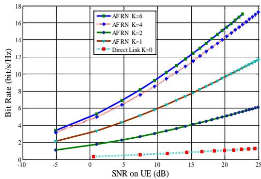
Figure (10) Bit rate and SNR enhancements using different relay nodes
