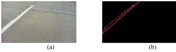
Figure 1: (a) Cement road with lane mark, (b) lane mark identified on Figure 1.(a)
