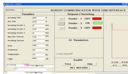
Fig 10: shows with GSM when the feeder2 is ON, in the green colour and the corresponding values are displayed.
