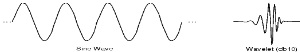
Fig1(b) . Comparison between Sinusoidal wave and a Wavelet
