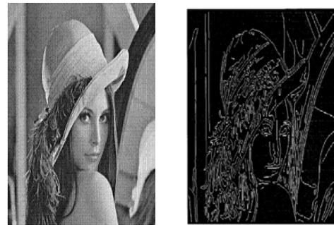
Fig. 2. (a) Original Lena Image; (b) After Averaging and Edge Detection Templates by employing RK-Embedded Heronian Mean.
