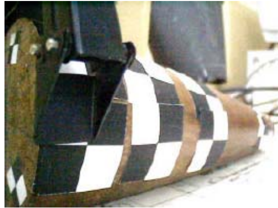
Fig.5.3a. End effector is at point 7 mm from the centre of the frustum
