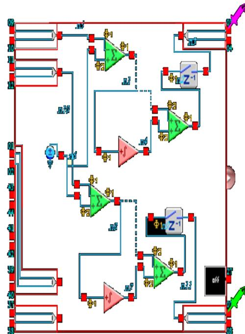
Figure 5 PI Controller FPAA Circuit
