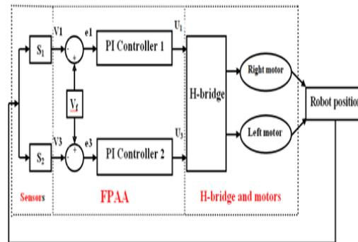
Figure 4 Path Tracking Robot Control System Block Diagram
