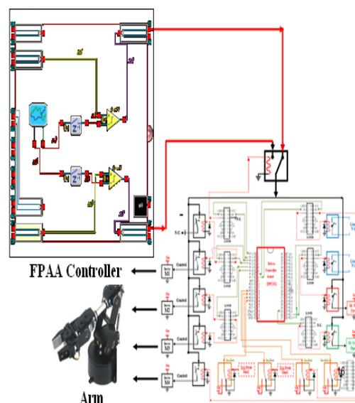
Figure 7 FPAA controller circuit used to control the arm motion
