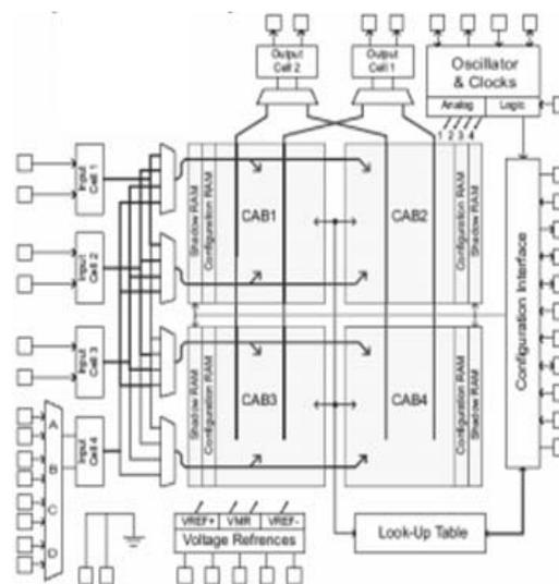
Figure 2 Block diagram of AN221E04 FPAA
