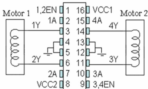
Figure 3 H-Bridge circuit L239D for DC motors
