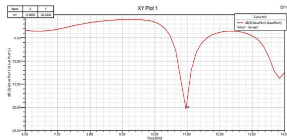
Figure (3) Return loss curve
