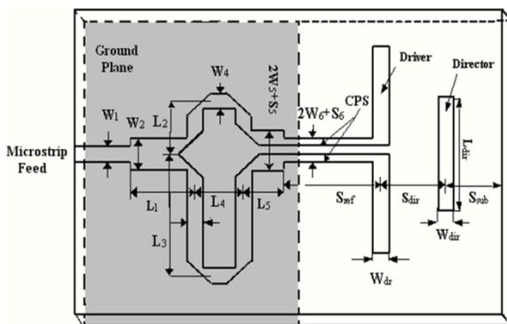
Figure (1) schematic diagram of uniplanar quasi yagi antenna
