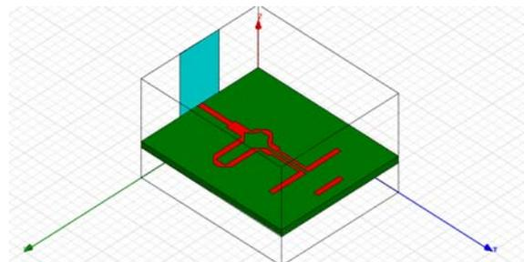
Figure (2) Ansoft model of quasi yagi antenna
