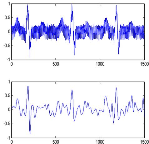
Fig.6. Recorded ECG and processed ECG using wavelet
