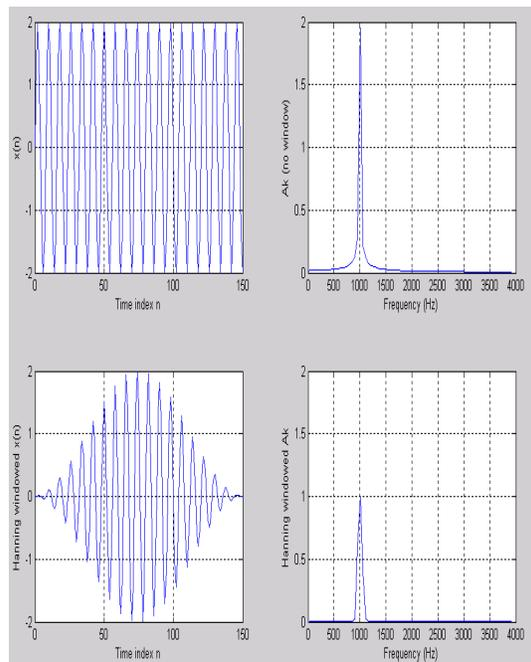
Fig.2. Hamming window frequency response
