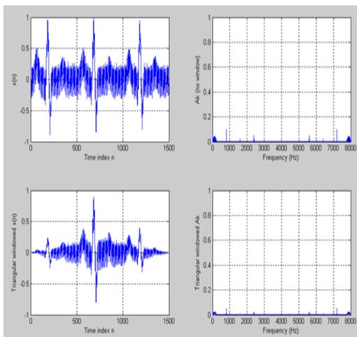
Fig.5. frequency response of noisy ECG
