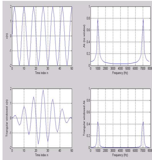
Fig.1.Triangular window frequency response
