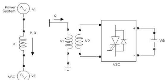
Figure 1. Schematic representation of STATCOM
