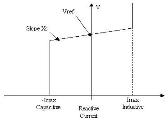
Figure 2. V-I characteristics of STATCOM
