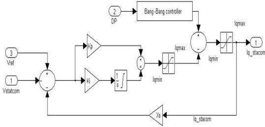
Figure 3: STATCOM model with Combined conventional PI – Voltage Regulator and Bang-Bang Controller block diagram
