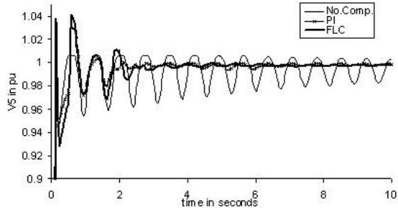
Figure 11: Voltage at Bus - 5 for 3-Ph Short-circuit at Bus - 7
