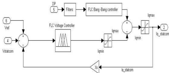
Figure 4: STATCOM model with Combined FLC Voltage Regulator and FLC Bang-Bang controller block diagram
