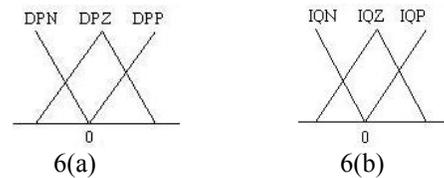
Figure 6: (a) Input membership function (DP) and (b) Output membership function (IQ) for FLC bang-bang controller
