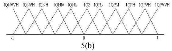
Figure 5: (a) Input membership function (Ve) and (b) Output membership function (IQ) for FLC Voltage regulator
