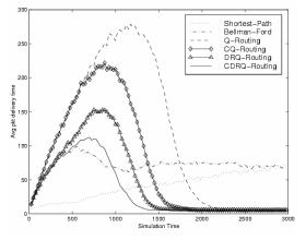
The main deficiency of Q-Routing was converging to optimal policy when network load decreases from high to low. As shown from the above figure CDRQ-Routing almost overcomes this problem.
