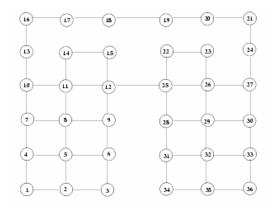
Above shown 6\*6 irregular grid was used. There are only two links to connect 18 nodes of one part of network to those of the other. Different experiments were performed by using shortest path nonadaptive algorithm, distributed Bellman Ford, Q-Routing, CQ-Routing, DRQ-Routing and CDRQ-Routing.
