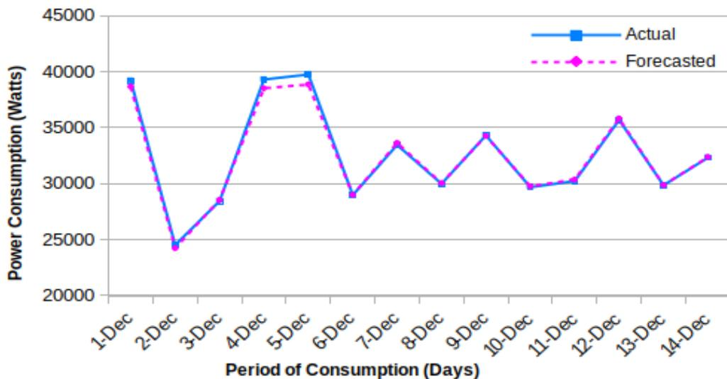
Figure 3: Prediction of power consumption using optimized SVR-ABO
