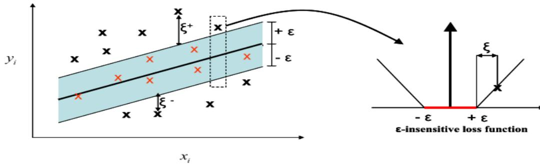
Figure 1: Slack variables and error tolerance of SVR
