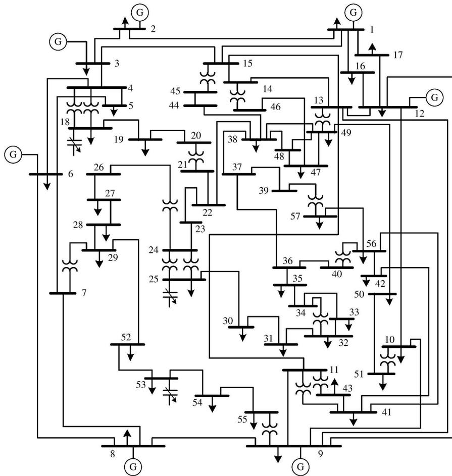
Figure 4: Single Line Diagram of IEEE 57-Bus Test System
