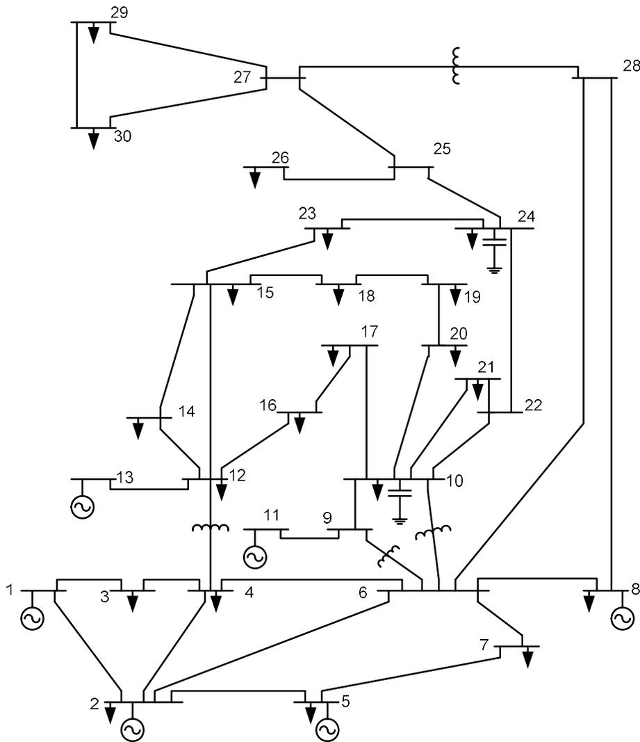
Figure 2: Single Line Diagram of IEEE 30-Bus Test System
