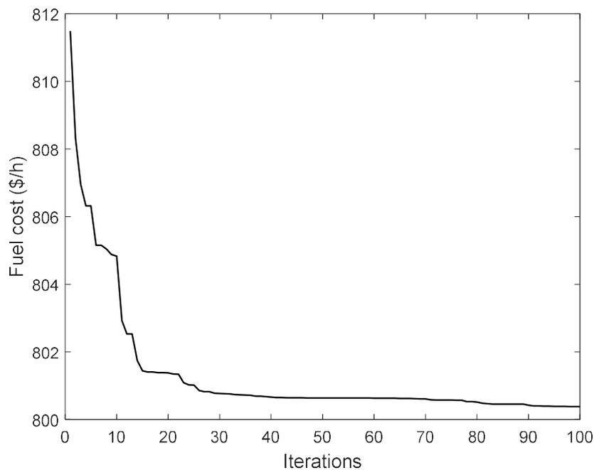
Figure 3: Cost Convergence Characteristics for IEEE 30-Bus Test System
