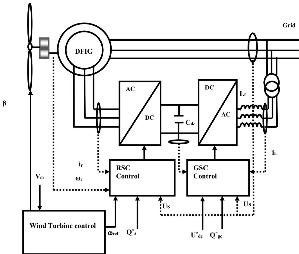
Figure.1. Configuration Of A DFIG Wind Turbine System
