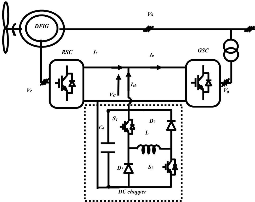
Figure 2 : The main circuit of DFIG wind power system based on SMES.
