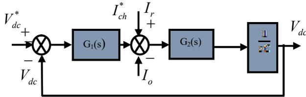
Figure . 4. Block diagram of the dc-link voltage control.
