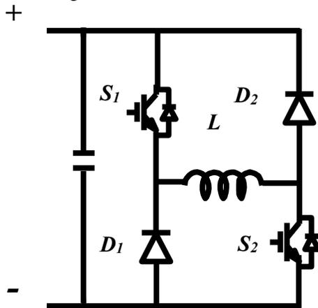
Figure 3. The DC-DC converter connecting the SMES to the DC-link
