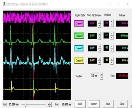
Figure 14: Butterworth filter input and output ECG
