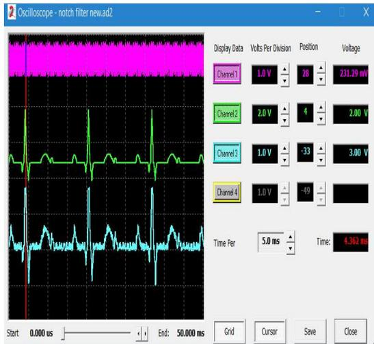
Figure 3: The corrupted ECG signals
