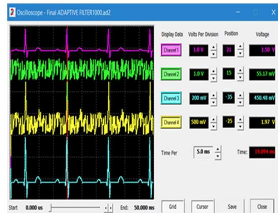
Figure 15: Adaptive filter input and output ECG signals
