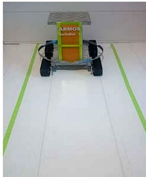
Figure 5: Configuration of the tests for straight-line forward motion of the robot
