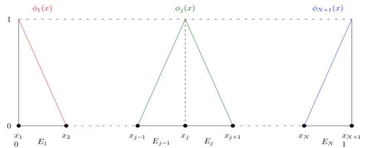
Fig 2. Piecewise smooth linear basis functions  $\varphi_1, \varphi_j, \varphi_{n+1}$  [13].
