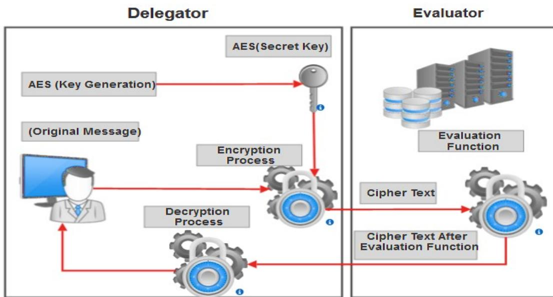
Figure 3: FHE Over AES Symmetric Key
