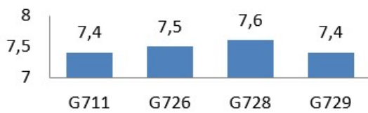
Figure 9: Total network delay (ms) by codec type
