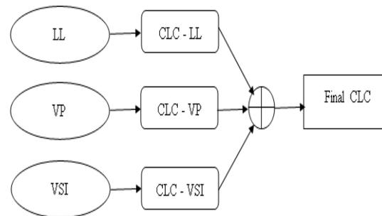
Figure 1: Parallel operated composite logic criteria system
