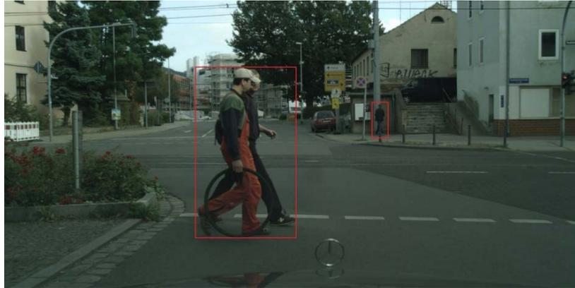
Figure 6: Example of Pedestrian Detection Results with Low NMS Threshold.
