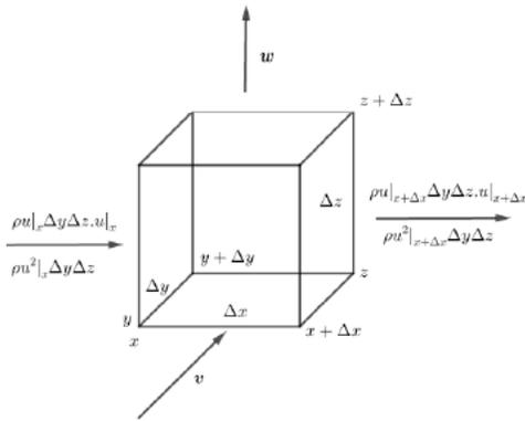
Figure 4: Illustration of the Balance Momentum
