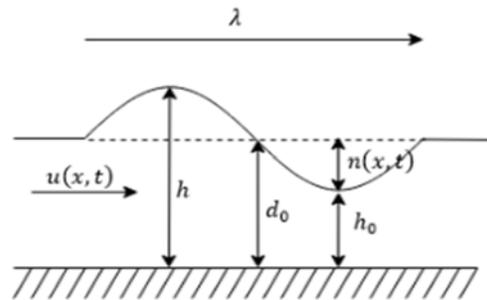
Figure 1: Shallow Water Equation Phenomenon
