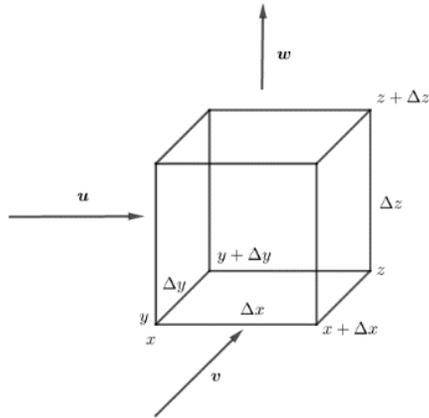
Figure 3: Illustration of Element Volume
