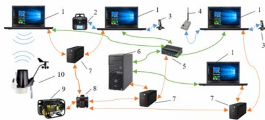
Figure 7: Interconnection Of Operator Workplace Equipment
