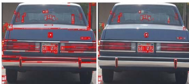
Figure 3: MSER Results on Grayscale Channel of Image, (a) Original MSER Results, (b) MSER Results after Filtering Out False Character Candidates.
