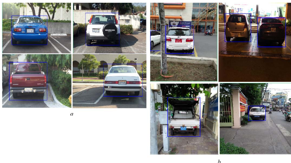
Figure 2: Examples of Vehicle Detection on Two Test Datasets, (a) Caltech Cars Dataset, (b) Collected Dataset. Vehicle Regions with Blue Rectangles are Extracted for Next Step.
