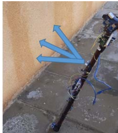
Figure 22: Detect Forward Obstruction Using Ultrasonic-1.
