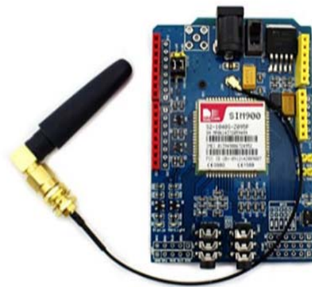
Figure 11: The SIM900 GSM/GPRS [13].
