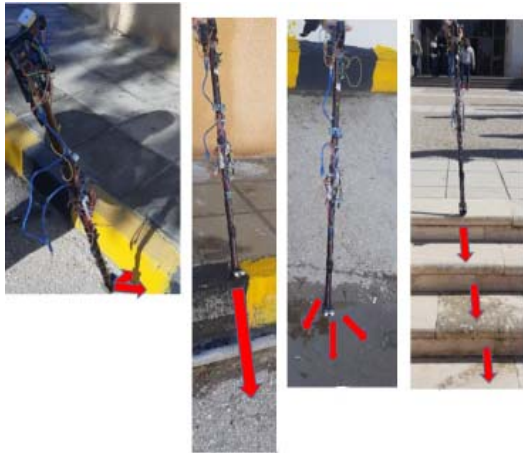
Figure 23: Detect Obstructions Below The Ground Level Using Ultrasonic-2.
