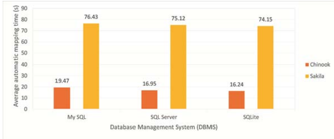
Figure 7. The Average Automatic Mapping Time In Seconds For Chinook And Sakila Databases
