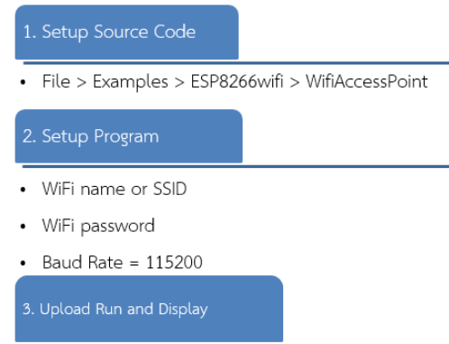
Figure 10: The Procedures of NodeMCU, Client and Website Connection
