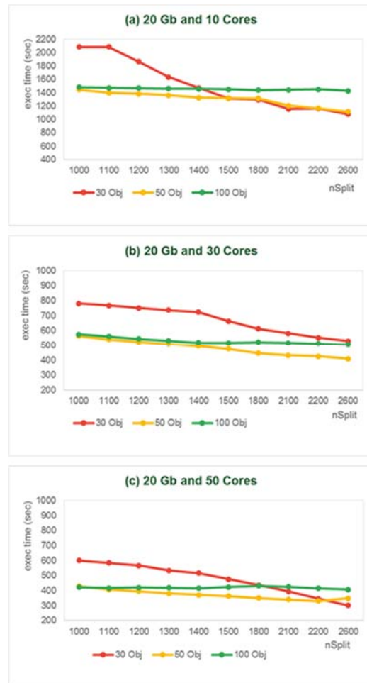
Figure 24. Time execution of Spark BDRT 20 Gb data on 10 machines and 3-5 cores.
