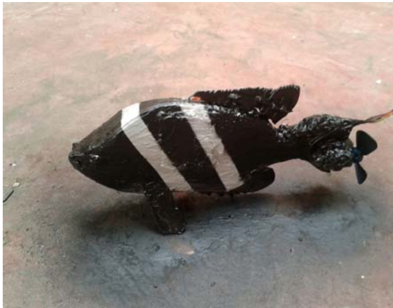
Annex 6. total waterproofing of the fish robot.
