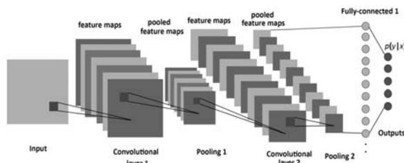
Figure 3: The general architecture of convolutional neural networks
