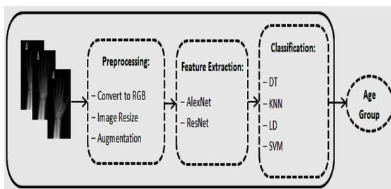
Figure 1: The block diagram of the proposed bone age assessment system
