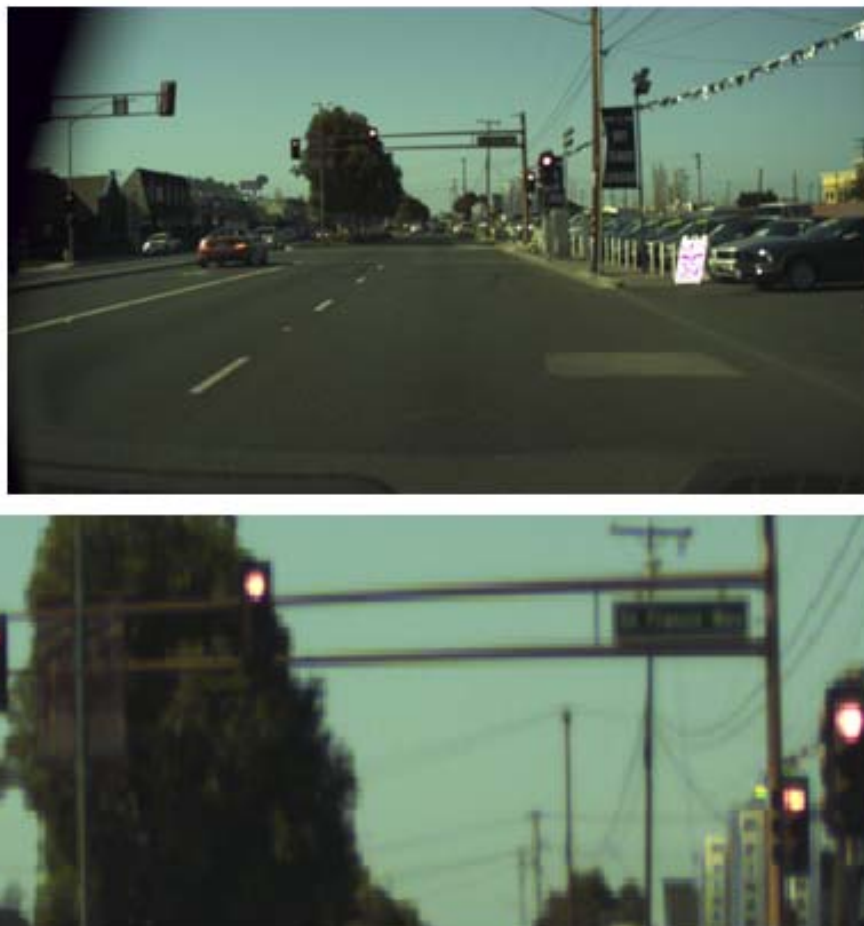
Figure 1: Traffic Light Instances (Bottom) in Traffic Scene Image (Top). Traffic Light Instances Have Resolution of about 8 \times 14 Pixels, and Original Image Has Resolution of 1280 \times 720 Pixels.
