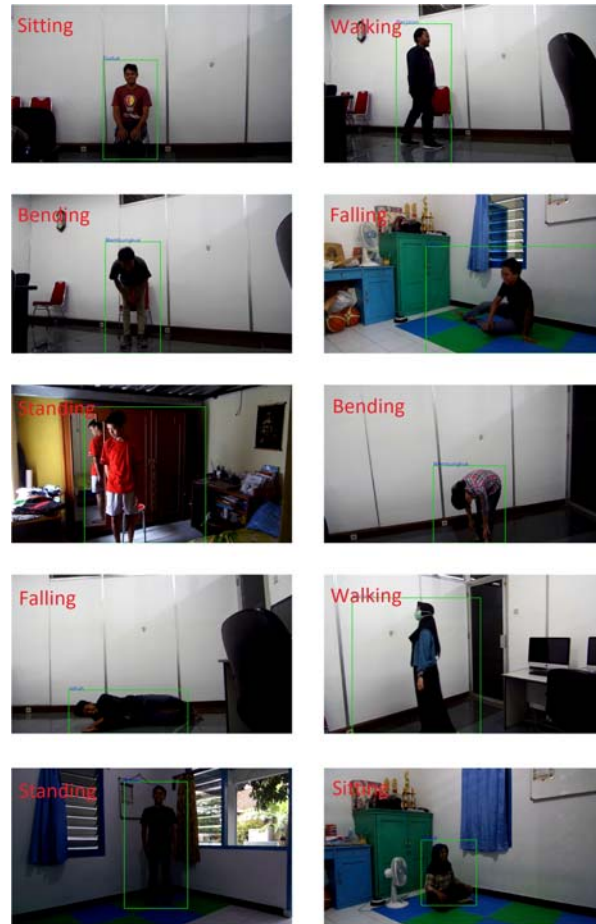
Figure 6: The sample results of action recognition from testing videos with detected area is indicated by green bounding boxes.
