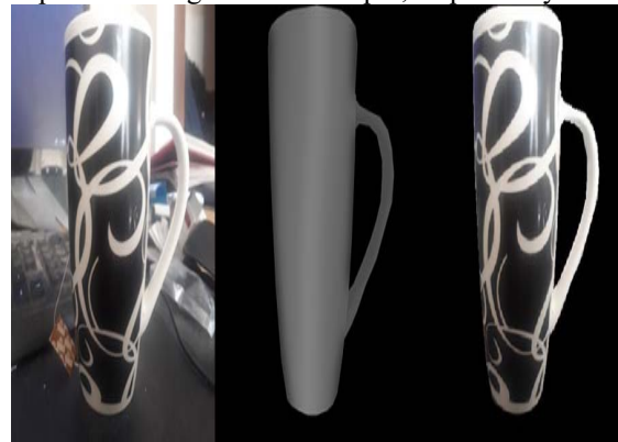
Figure 17: Object of interest on the left, manually-processed depth map on the middle, and the segmented image on the right.
