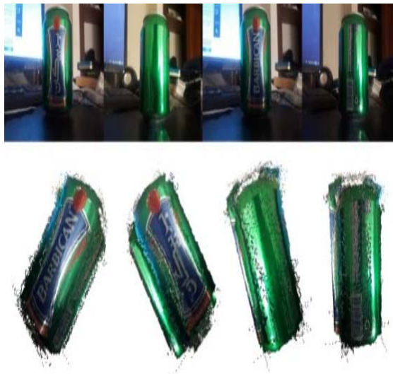
Figure 19: Input images of the 4-views case on top and the final reconstructed model on the bottom.
