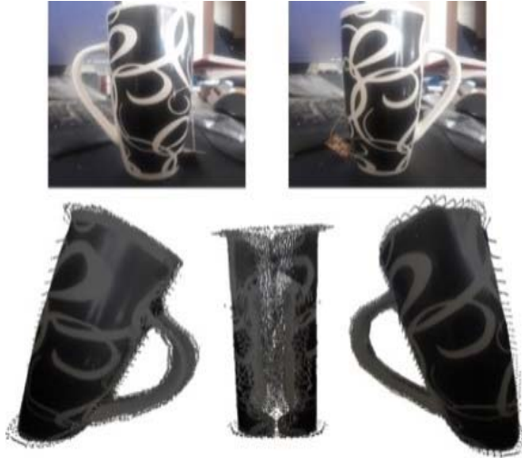
Figure 18: Input images of the 2-views case on top and the final reconstructed model on the bottom.
