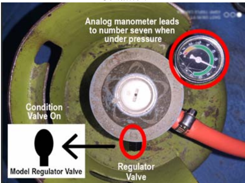
Figure 11: First Regulator with Valve Locking Condition
