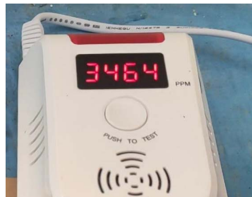
Figure 7: Detection Results from Combustible Gas Detector GD13MPX5700
