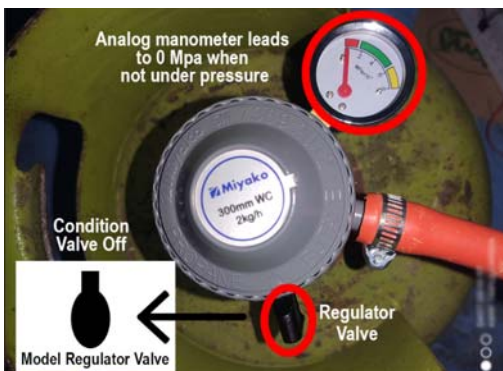
Figure 12: Second Regulator with Valve Condition Not Locking
