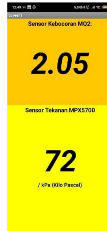
Figure 15: Smart Regulator Application of Gas Leak Detection and Gas Monitoring based on IoT
