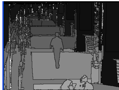
Figure 2: Illustration of watershed segmentation on weighted gradient image.
