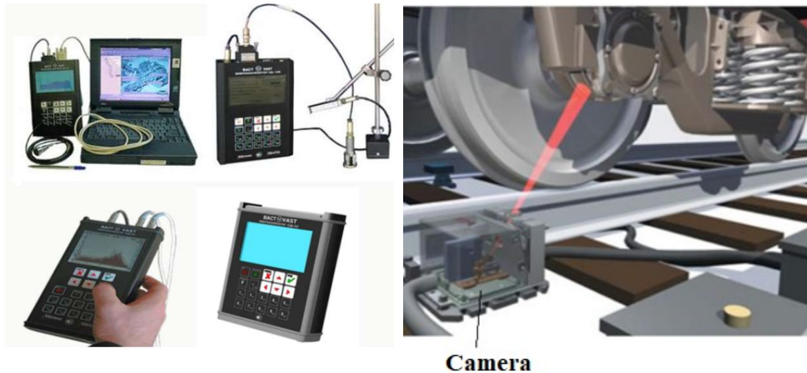
a) small-sized devices for non-destructive vibration control and diagnostics of nodes and aggregates
