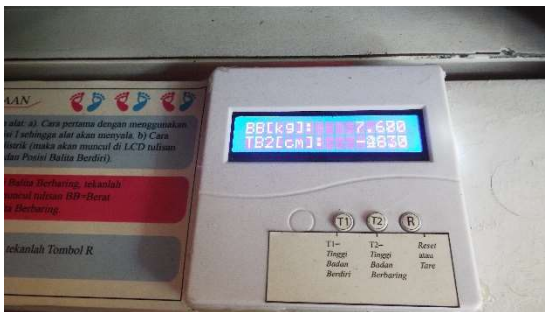
Figure 18. The display of LCD when doing the weight measurement of under five-year-old children directly on the system
