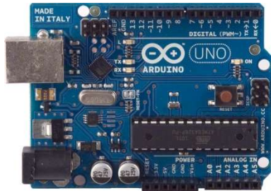
Figure 6: Arduino Uno R3
