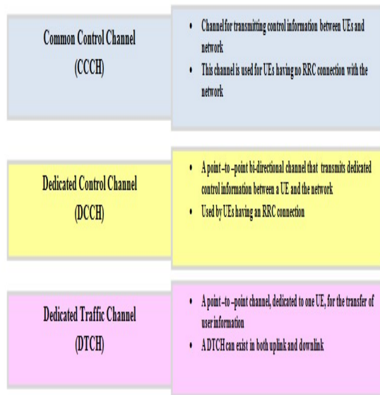
Figure 7: LTE Uplink Logical Channels
