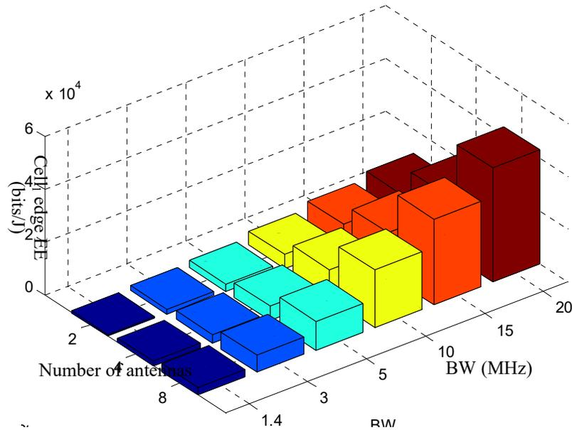
Figure 8: Energy efficiency versus different BW values for different number of antennas at  $P_{tx\_eNB1} = P_{tx\_eNB2} = P_{tx\_eNB3} = 46$  dBm and at the lowest SINR (at edge of cell)
