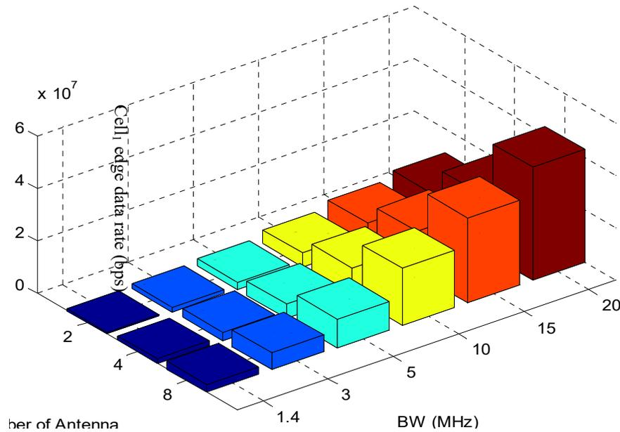
Figure 6: Data rate versus different BWs values for different number of antennas at  $P_{tx\_eNB1}=46$  dBm and the lowest SINR (at edge of cell<sub>1</sub>)
