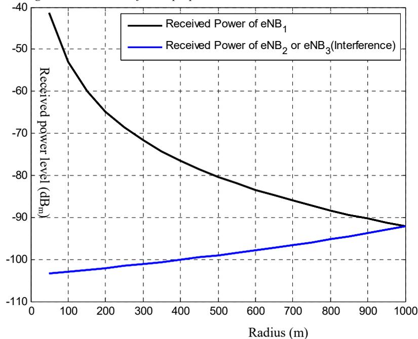
Figure 4: Cell radii versus received power level at  $P_{tx\_eNB1} = P_{tx\_eNB2} = P_{tx\_eNB3} = 46$  dB<sub>m</sub>
