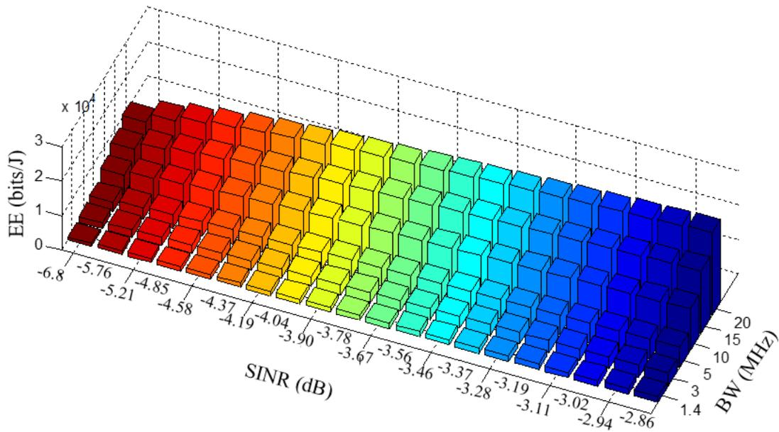
Figure 7: Energy efficiency versus different SINR values for different BWs at  $P_{tx\_eNB1} = P_{tx\_eNB2} = P_{tx\_eNB3} = 46$  dBm and  $N_{Ant}=2$
