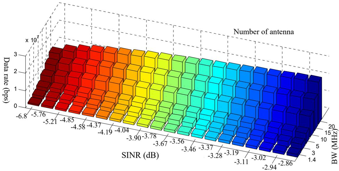
Figure: 5 Data rate versus different SINR values for different BWs at  $P_{tx\_eNB1}=46$  dB<sub>m</sub> and  $N_{Ant}=2$
