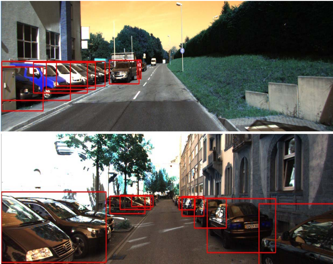
Figure 9: Undetected Vehicle Due to Small Size, Heavy Occlusion or Truncation of The Vehicles.
