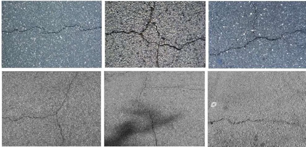
Figure 5: Example Images in CRACK500 Dataset (First Row) and CrackTree Dataset (Second Row).
