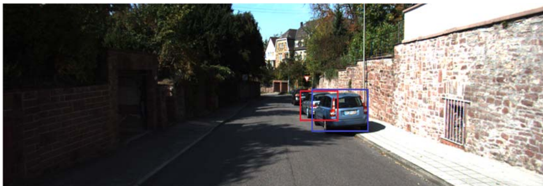
Figure 2: Example of Traditional NMS Algorithm. Front Vehicle May Be Removed with High Probability by The Traditional NMS Method
