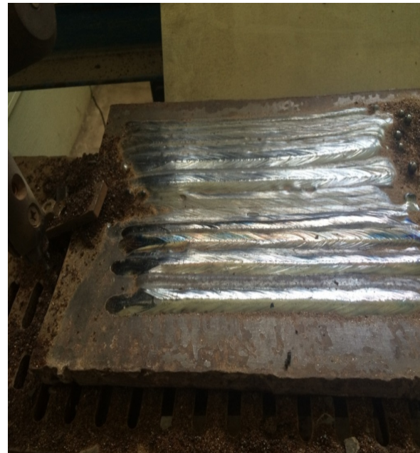
Figure 8 : First layer of weld metal
