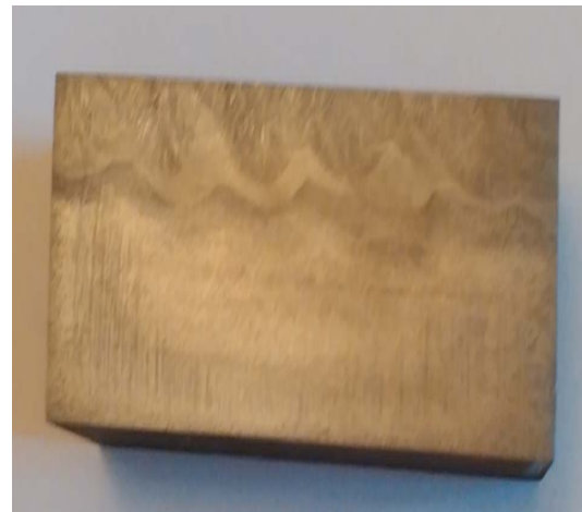
Figure 12 : Sample without cracking after plastic deformation
