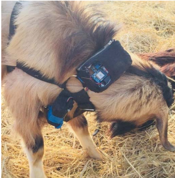
Figure 3: Fully assembled Smart Collar worn on the goat.
