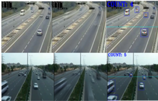
Figure 3 (a) Input video frame (b) Multi-cue color background subtracted image (c) Vehicles Identified and counted in Two-way roads in Highway roads and City roads in India
