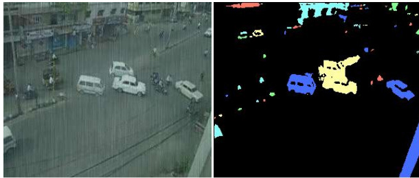
Figure 7(b). The results of the algorithm which removes the rain streaks from the input image and identified the moving vehicles.
